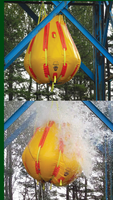
5 tonnes parachute air lift bag, before and during type testing. Recorded peak load of 51 tonnes, giving 10:1 safety factor.
